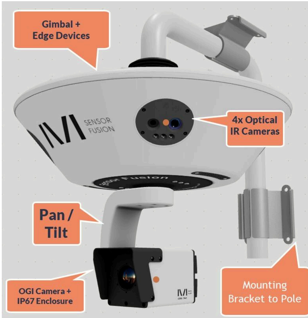
Figure 1. External view of the Minerva Platform, the primary physical component of the CleanConnect LeakFinder system.
